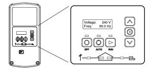
The RDC2 controller provides integrated control for the generator set, Kohler<sup>®</sup> Model RXT transfer switch, programmable interface module (PIM), and load control module (LCM).
